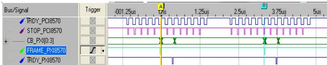
Figure 5. Host PCI bus signals (PCI8570) and extension bus signals (PXI8570)
