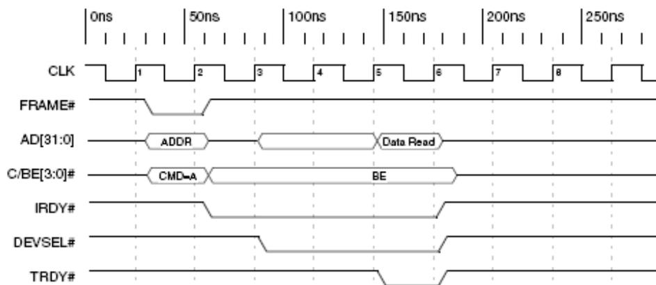
Figure 3. PCI signals for a single read operation.
