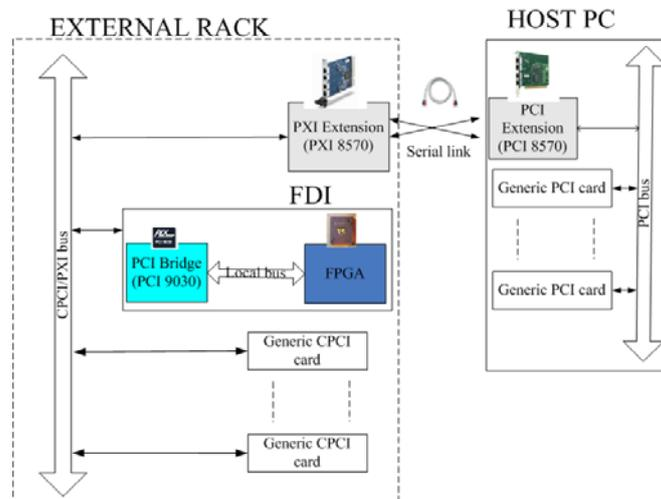
Figure 1. Architecture of the PXI-based communication system of the FDI.
