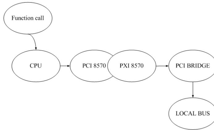
Figure 2. Procedure of the initiator-target chain of the FDI PXI communication.
