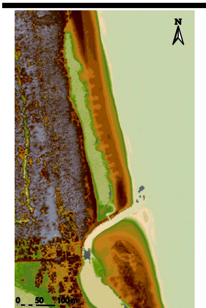
Figure 5. Recent Lidar survey of the Bevano barrier (February 2009) showing the washover fans.
