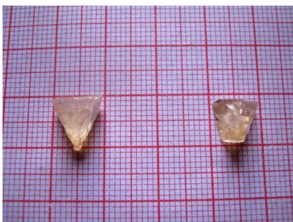
Fig. 1. Photograph of as grown crystals of L-tyrosine hydrochloride.
