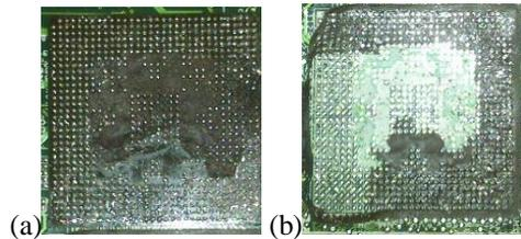
Fig. 3. Typical cut from a home produced BGA/Stencil/PCB interconnect showing cross-sections covered with the stencil on the BGA side (a) and on the PCB side (b).
