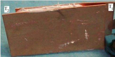
Fig. 4. Specimen used to measure the thermal conductivity of a sample (shown in white) of a non-solid material sandwiched between two copper plates.
