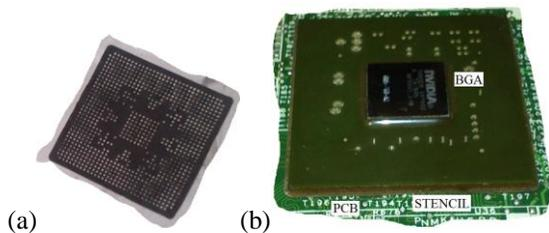
Fig. 1. Typical stencil (a) and typical reworked interconnect showing the BGA on top of the stencil (b).
