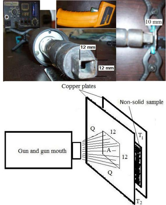
Fig. 5. Soldering Heating Station Gun and IR Thermometer (shown in orange) and set-up showing the specimen.
