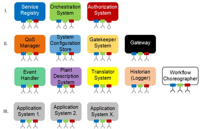
Fig. 5. Core Systems of the Arrowhead Framework
