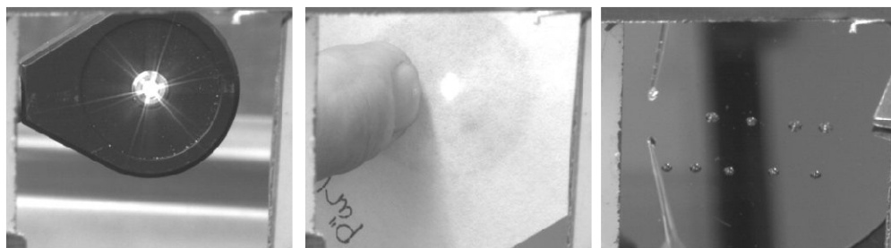
Figure 2. Calibration fiber, laser spot and application of 1 \mu\text{l} droplets on silicon wafers.
