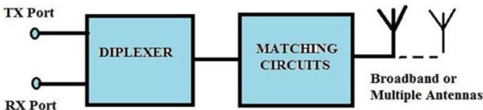
Fig. 23.6 Block diagrams of a traditional diplexer antenna system [27]
