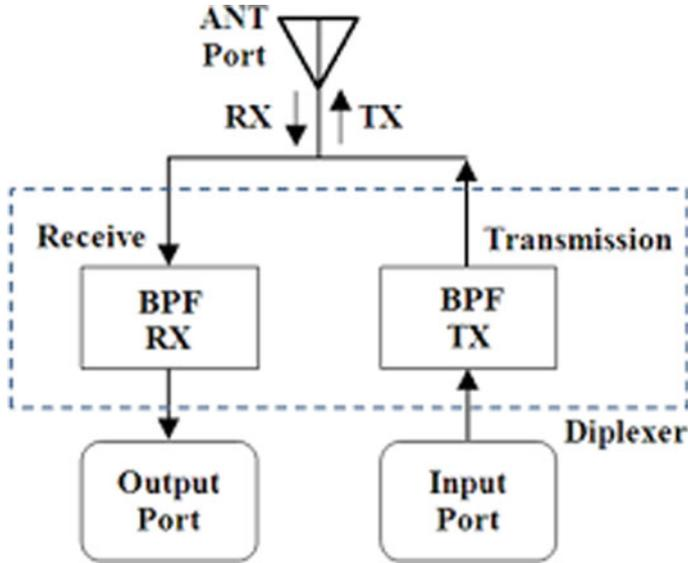
Fig. 23.7 Diplexer working for transmission and receiving antenna [24]
