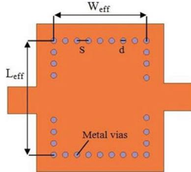
It also combines the advantages of microstrip (low cost, easy fabrication, compact size, low weight) and metallic waveguide (low loss, complete shielding and high power handling capability) [40]. Figure 23.5 depicts a typical SIW structure.
