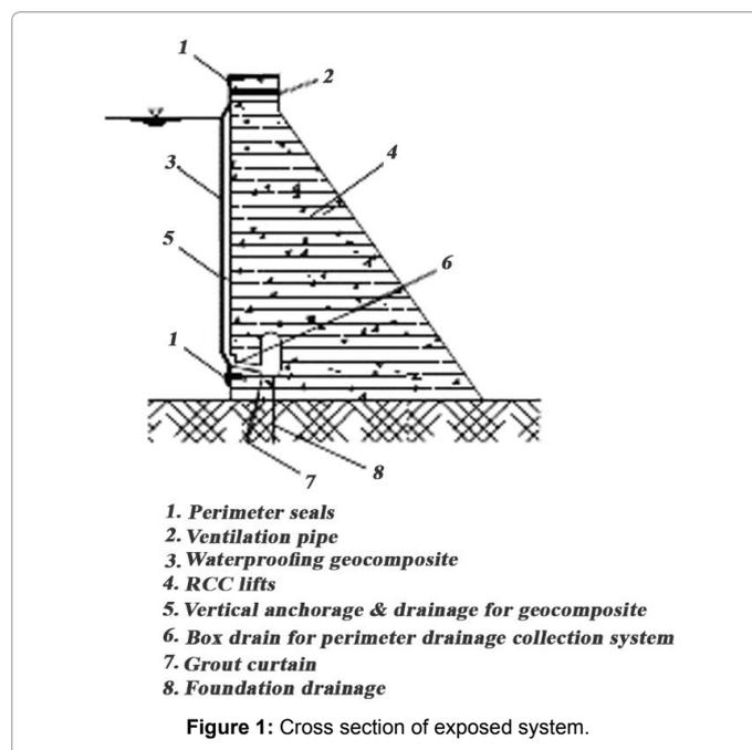
Figure 1: Cross section of exposed system.
