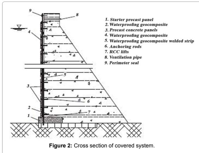
Figure 2: Cross section of covered system.
