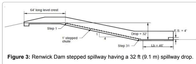
Figure 3: Renwick Dam stepped spillway having a 32 ft (9.1 m) spillway drop.
