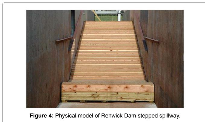
Figure 4: Physical model of Renwick Dam stepped spillway.
