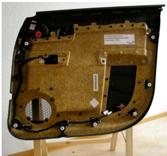
Figure 6.12 Car door trim fabricated from hemp fiber–reinforced polyethylene [16].
