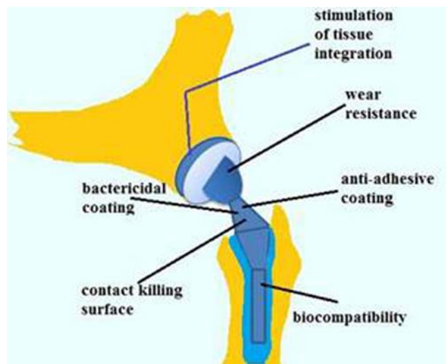
Figure 11.1 Multifunctional surfaces of an implant.
