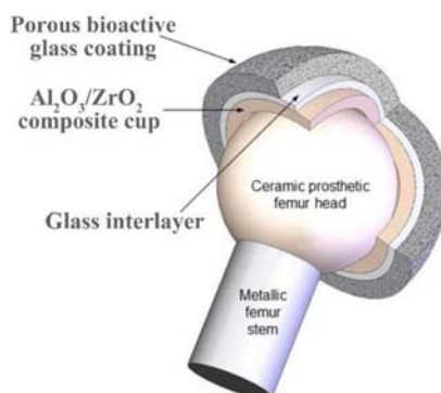
Figure 6.5 Usage of \text{Al}_2\text{O}_3\text{--ZrO}_2 composites in hip prosthesis [3].
