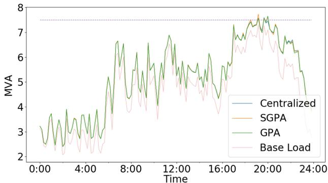
Fig. 6: Substation loading at different time slots for centralized, GPA and SGPA. The horizontal (purple) dashed line represents the rating of the substation transformer.
