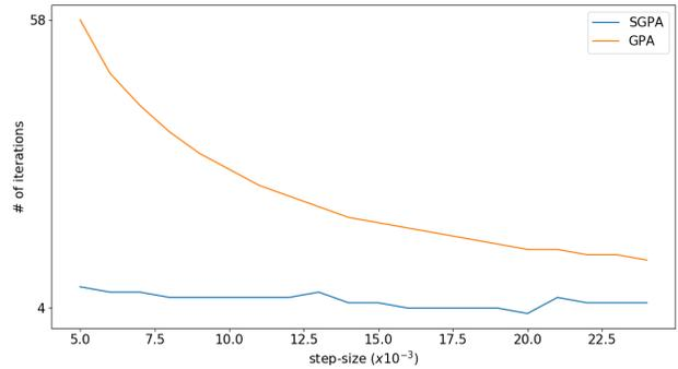
Fig. 12: 95% convergence analysis of SGPA and GPA for a specific time slot (7:00 pm) for scenario A. Here the initial points for both algorithms are same
