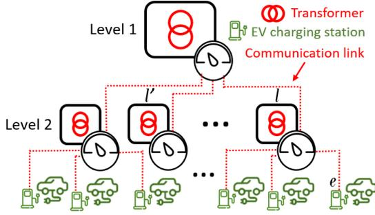
Fig. 2: The logical view of a radial distribution network.
