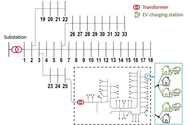
Fig. 1: The one-line diagram of a radial distribution network. The network is divided into primary (Nodes 1-33) and secondary feeders (an example shown in the dashed-box).
