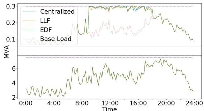
Fig. 9: Transformer loading over one day using centralized, LLF and EDF. The top plot is for a distribution transformer and the bottom one is for the substation transformer.
