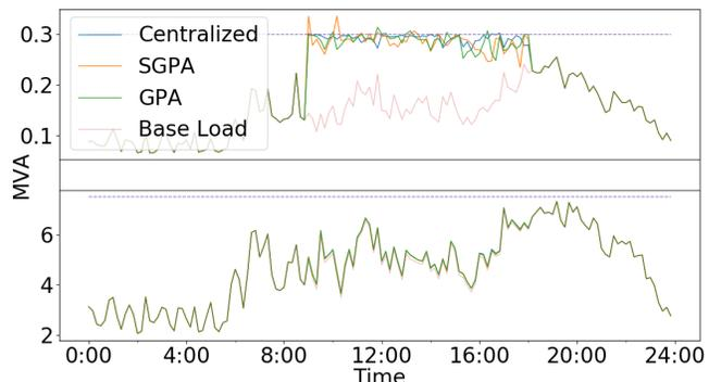
Fig. 8: Transformer loading over one day using centralized, SGPA and GPA. The top plot is for a distribution transformer and the bottom one is for the substation transformer.
