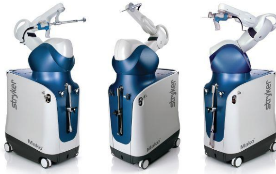
Figure 2.10. MAKO ® Robotic-Arm Assisted Surgery.
