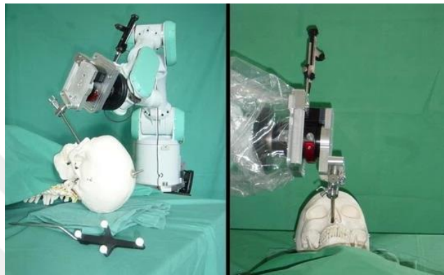
Figure 2.17. The robot arm PA10–6c with Strauß et al.’s designed holder mechanism (Source: Strauß et al., 2007)
