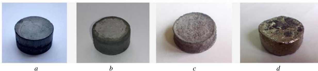
Fig. 6. Appearance of samples (TiH_2)_{40}Zr_{40}Ni_{20} : a – initial after pressing; b – No. 4a after annealing in vacuum at T = 800 °C; c – No. 4b after annealing in vacuum at T = 870 °C for 2 h; d – No. 4c after annealing in vacuum at T = 800 °C + SHS on EBM
