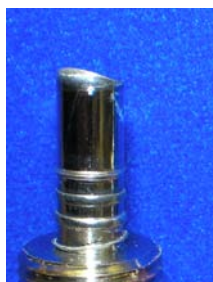
Fig. 7 Double Bridgman after pressurisation, showing the ripple effect of the lead seals.
