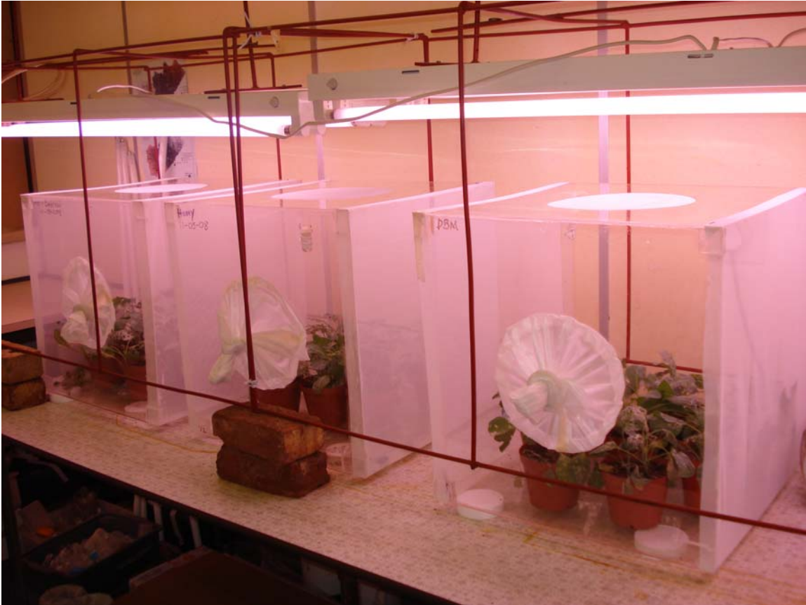
Figure 2.1: Ventilated insect rearing cages (53 × 53 × 53 cm) with four sides made of clear Perspex, while two opposite sides were entirely covered with nylon mesh to allow free flow of air through the cages. The rearing cages were directly illuminated by a number of FLUORA L58W/77 fluorescent tubes (OSRAM, Germany) which provided adequate light to support the photosynthetic process in the cabbage seedlings.
