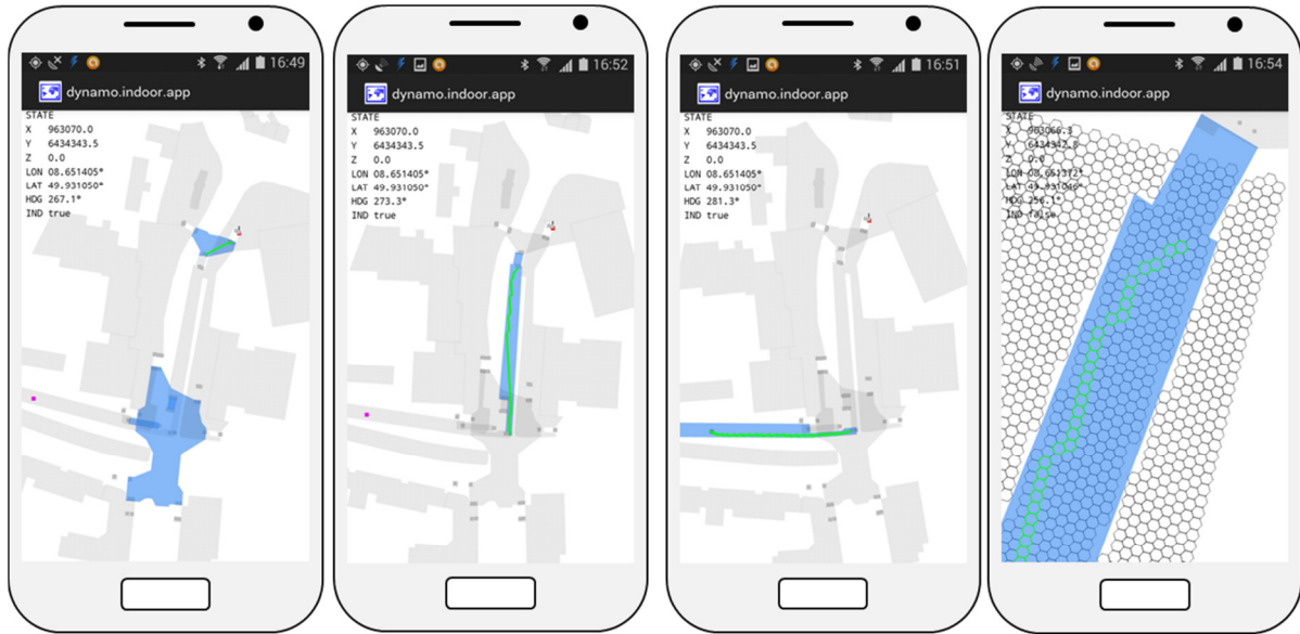
Figure 9 Indoor route segments as result of A* pathfinding in hexagonal grids on multiple floors of a subway interchange station.
