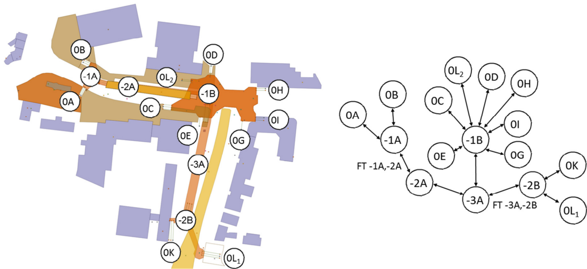
Figure 7 Geo-referenced model of a railway and subway station with corresponding topological 2.5D graph of floors (nodes) and floor transfer connectors (edges).
