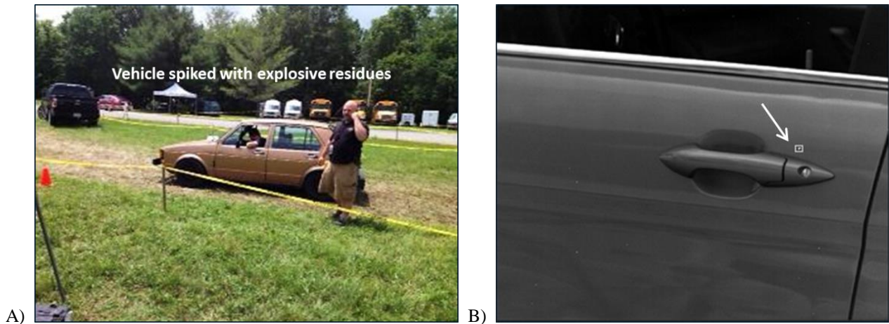
Figure 2. Example vehicle checkpoint scenario. A) Digital Image of a vehicle spiked with explosive residue; B) SWIR detection image shows a fingerprint transfer of an explosive. An arrow was added to the SWIR image to emphasize the detection.
