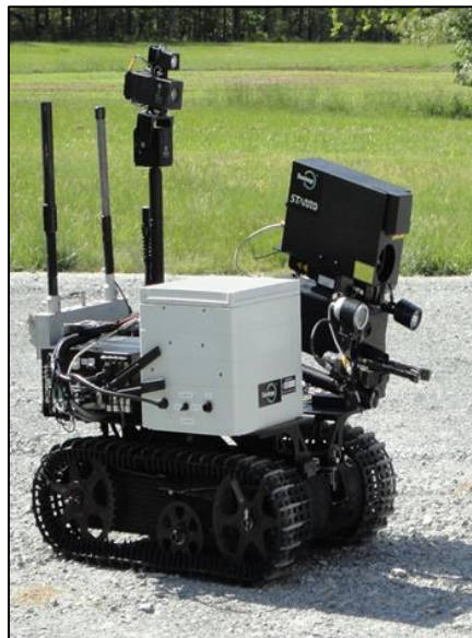
Figure 4. STARR sensor during field testing.
