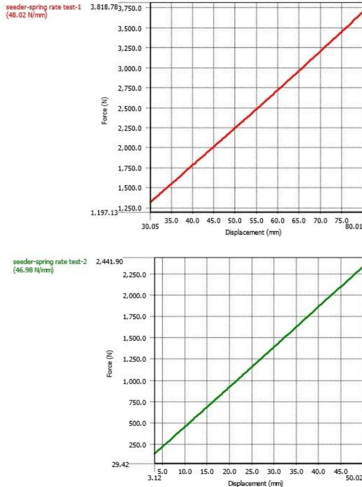
**Figure 7. Forward spring rate test 1, 30mm,3.12mm preload, respectively**
