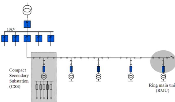
**Figure 2: Traditional Distribution Radial Network**
