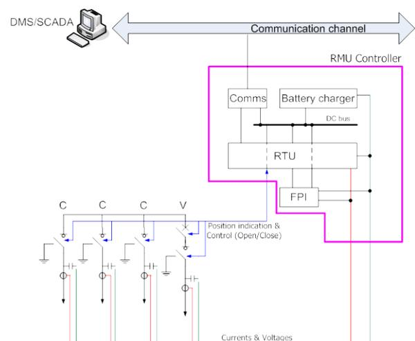
Figure 4: Remote monitoring and control of an RMU
