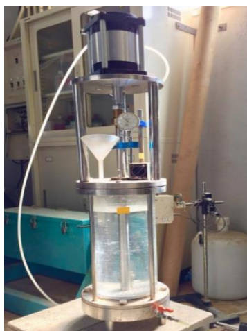
(b) Picture Figure 1 Rigid wall permeability test apparatus
