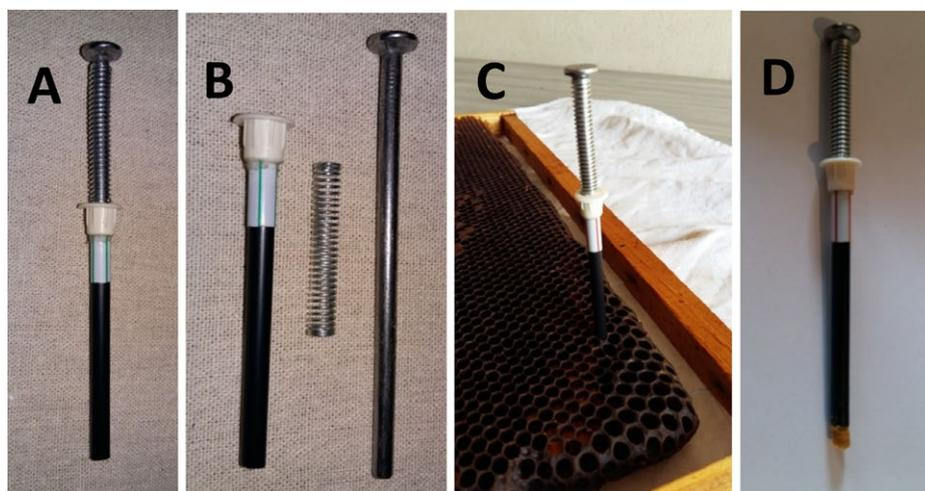
**Figure 2.** (A) The ready assembled beebread collector. (B) Components of the beebread collector: a small rigid tube; a plunger and a spring. (C) How to collect beebread: it is important to insert the beebread collector vertically into the cell. (D) A small pellet of beebread has been expelled from the beebread collector.
