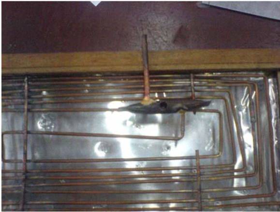
Figure 8. Bended pipes of the thermal collector.
