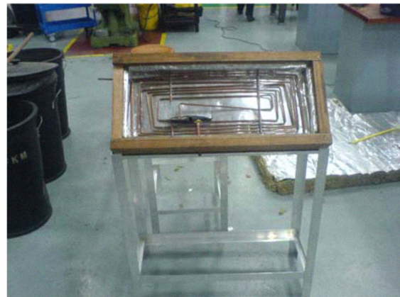
Figure 4. Construction of the Thermal collector
