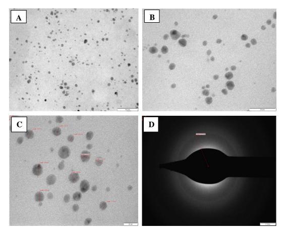
Figure 2: TEM analysis of generated silver nanoparticle using *Amaranthus oleracea* extract. A: Scale at 100 nm, B: Scale at 50 nm, C: Scale at 20 nm, D: SAD Pattern
