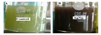
Figure 1: Visual observation of silver nanoparticles synthesized using *Amaranthus oleracea* leaf extract. A- Leaf extract of *Amaranthus oleracea* as a control, B- Reaction mixture of silver nitrate and leaf extract indicates the color change due to nanoparticle synthesis (brown color).
