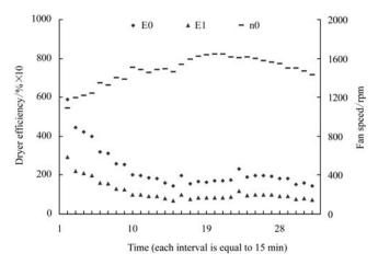
Figure 8 Efficiency and controlled fan speed variations with time
