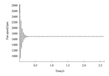
Figure 6 Response of system to 1700 rpm input
