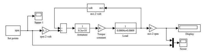
Figure 4 Fan simulation block diagram by MATLAB Software
