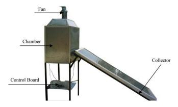
Figure 1 Experimental forced convection solar dryer
