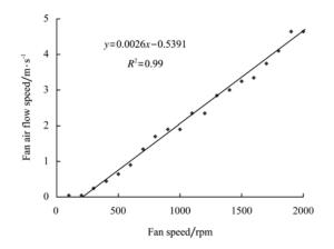
Figure 2 Variation of the fan outlet air speed with the fan speed
