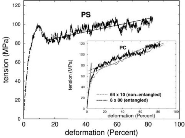
Fig. 3 – Simulated stress-strain dependence for a non-entangled model of PS ( $4 \times 160$  system) and two specimens of PC of different molecular weight (see inset), at  $T = 300$  K. Strain softening is absent for both entangled and non-entangled PC glasses. Straight solid lines represent the least-squares fit of the data in the strain-hardening regime and elastic regime (PC only).
