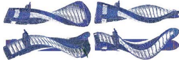
Figure 18. The first and the second coupled torsional and horizontal mode shapes (lateral and bird's view), 9415 TEU container ship.
