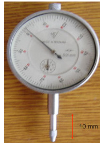
Figure 2 – Photograph showing the comparator clock (dial micrometric indicator) which was used with an adapted system for the microscope to measure the depth of the recess (only in the cases when the perpendicular axes of the microscope's view reached the bottom of the sinus).
