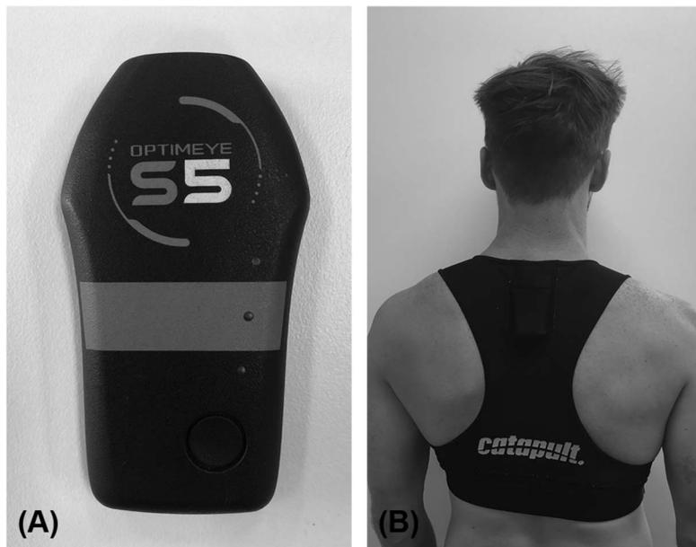
**Figure 3.** A) Catapult Optimeye S5 microtechnology unit (52 × 96 × 12 mm), housing a 10-Hz global navigation satellite system antenna, along with a triaxial accelerometer, gyroscope, and magnetometer, all sampling at 100 Hz; and (B) commercially manufactured, trunk-mounted, fitted vest displaying the placement of the microtechnology unit.
