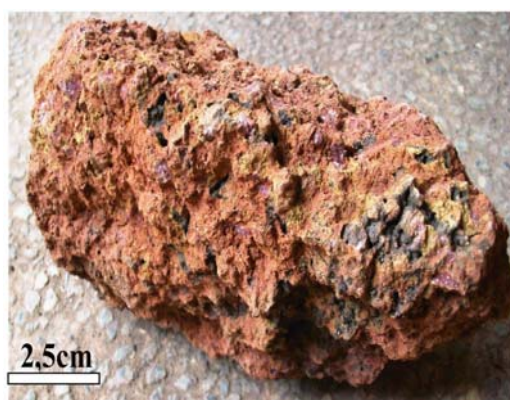
Figure 9. Nzie-Fonda bauxite Facies. Bauxitic material with massive vermiculate facies. It has void spaces.
