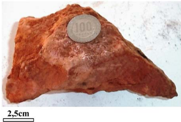
Figure 13. Kreu massive bauxite facies. Smooth massive bauxite devoid of cavities.
