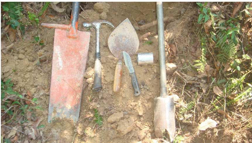
Photograph 2: Soil sampling equipment at a forest plot
