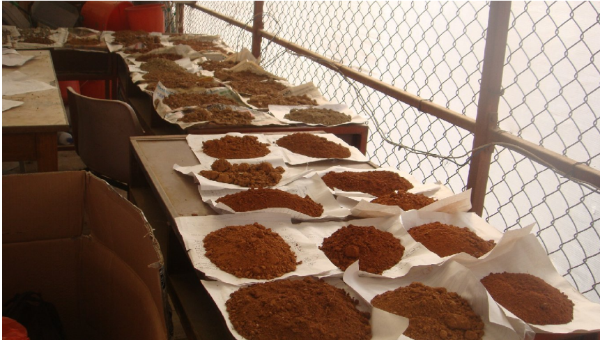
Photograph 4: Samples exposed to air drying before lab analysis
