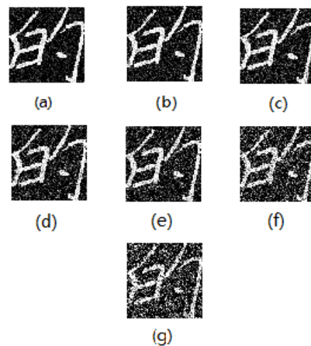
Fig. 6 Character 的 with increasing levels of added noise: (a)-(g) shows the intensities 10 – 70 respectively
