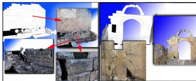
Figure 10: Adding orthphoto images as texture to the CAD model.
