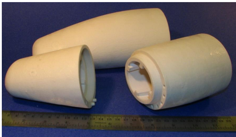
Figure 6 One piece and two piece socket molds created by 3D printing.
