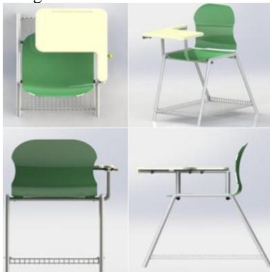
Figure 4. Different 3D views of the proposed student's chair as drawn by solid works software
