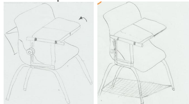
(a) Foldable desktop with book holder (b) Bag/book holder at lower desk at the back
