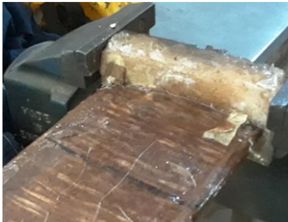
Figure 9 Fixture made from Sisal fibres and Epoxy Matrix attached to the root of the UAV wing to simulate the fuselage wing interface
