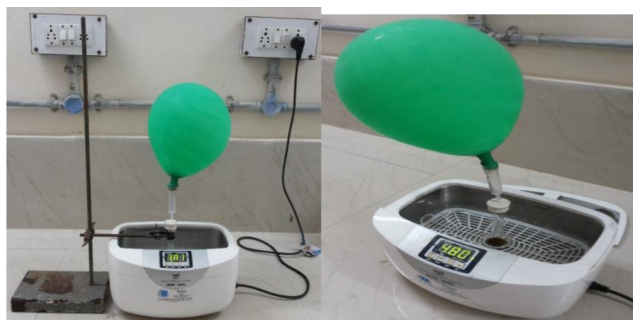
Figure 2: Ultrasonication setup to carry out the Buchwald's reactions under nitrogen gas environment.
