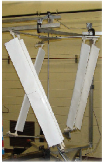
Figure 3: Vertical Axis micro Wind Turbine testbed the Georgia Tech 42" Wind tunnel.
