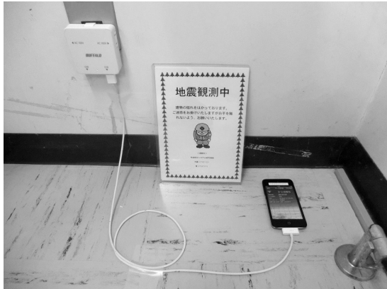
Fig. 14. Installation of “i-jishin.”
