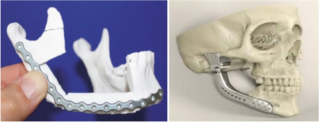
Fig. 8.13 3-D model print as a rehearsal and accurate measurement of the metallic plate and screws in a patient going to have right-sided hemimandibulectomy
