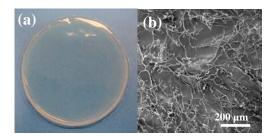
Fig.1: (a) Image of PVP-CMC film in the form of hydrogel, (b) cross-sectional view of freeze dried PVP-CMC hydrogel
