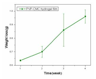
Fig. 5: Weight loss profile of PVP-CMC hydrogel film under compost environment.
