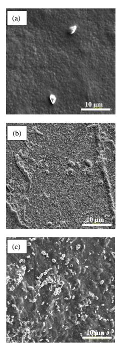
Fig. 4: SEM micrograph of PVP-CMC hydrogel film. (a) Initial and after (b) 2 weeks and (c) 4 weeks of bio-degradation.
