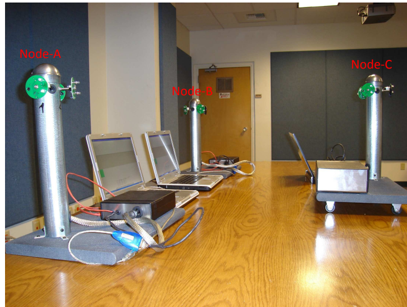
Figure 4.9: Indoor experiment setup: 3 laptops (collinear placement), each with a 3 transceiver optical antenna.
