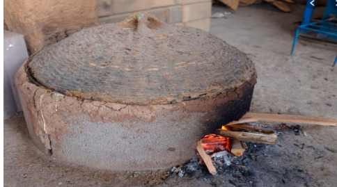
Fig. 5: Burayou mud Injera baking stove
