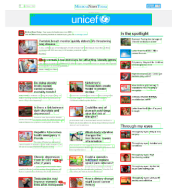
Figure 7.3: UI component detection on real web UI screenshots. Average processing time: 57s.
