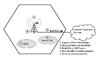
Fig 1. Backhaul and Radio are two choke points.
