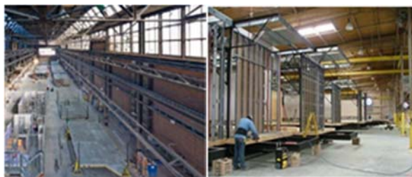
Figure-2. Three-dimensional or modular units are produced in a factory.
