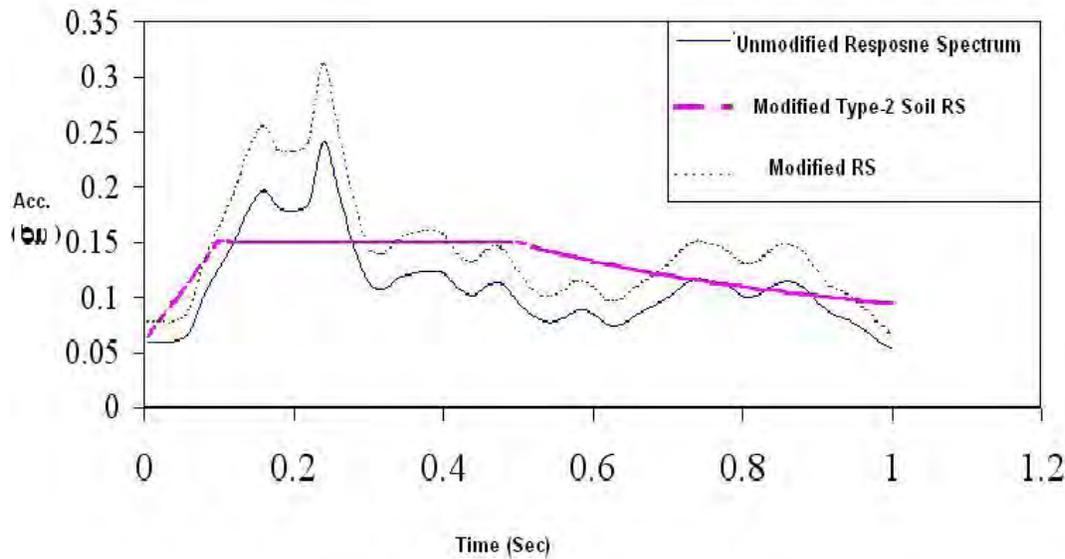
**Figure 10:** Response Spectra of Delijan's Cement Silo (Tabas EQ-Record)
