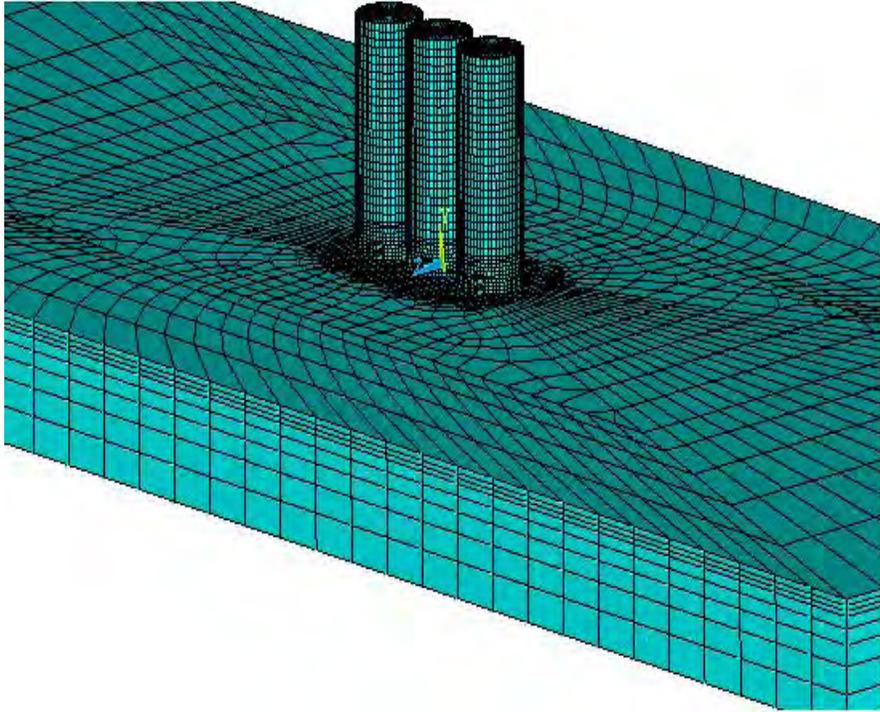
**Figure 4:** A Finite Element Model of three-Cell of Delijan’s Silo Structure and its Foundation
