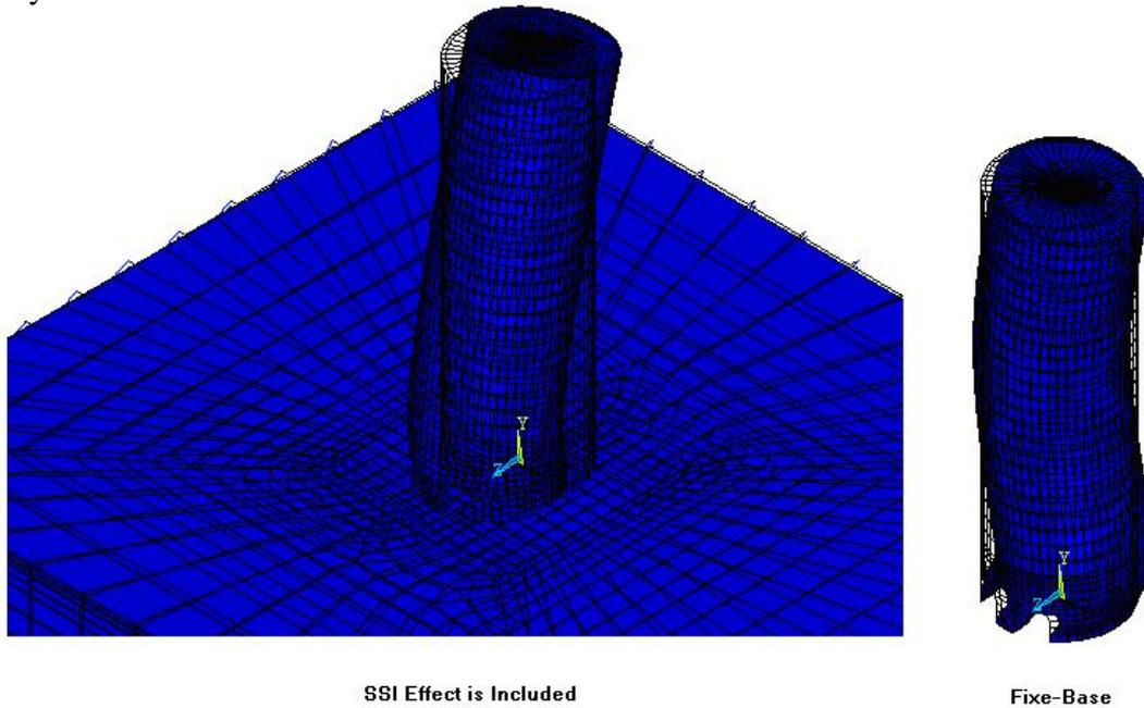
**Figure 8:** Shape of 7th Mode of Delijan's Cement Silo System (Tabas, El-Centro, Naghan)
