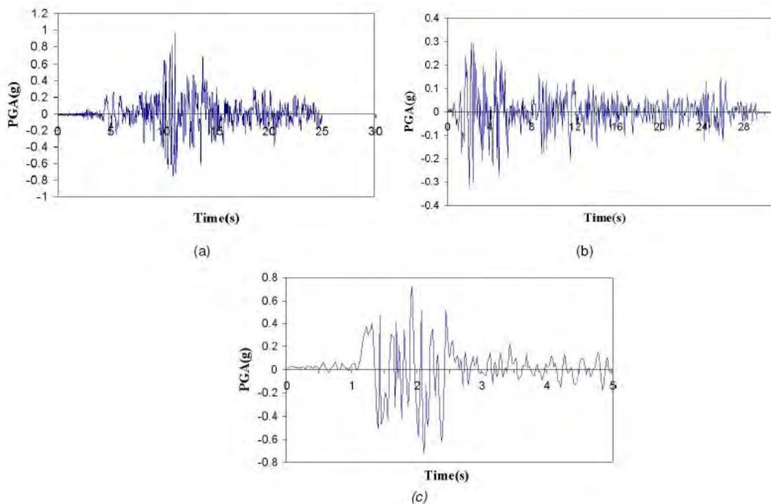
**Figure 6:** Seismic Records used for Analysis of Delijan's Cement Silo
