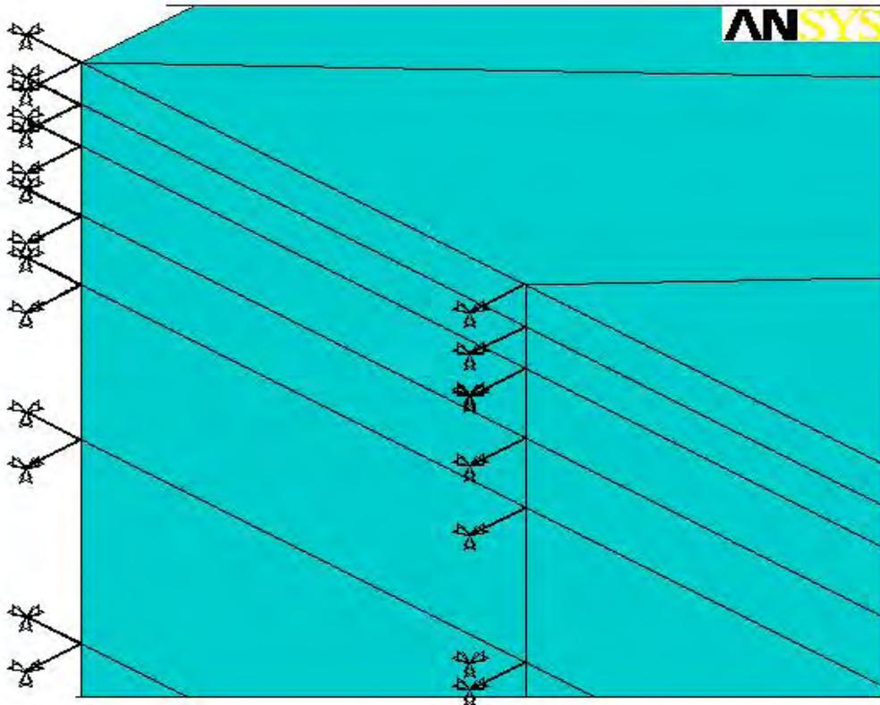
**Figure 5:** A Finite Element Modeling of Far-Field of Soil for Delijan’s Cement Silo Foundation
