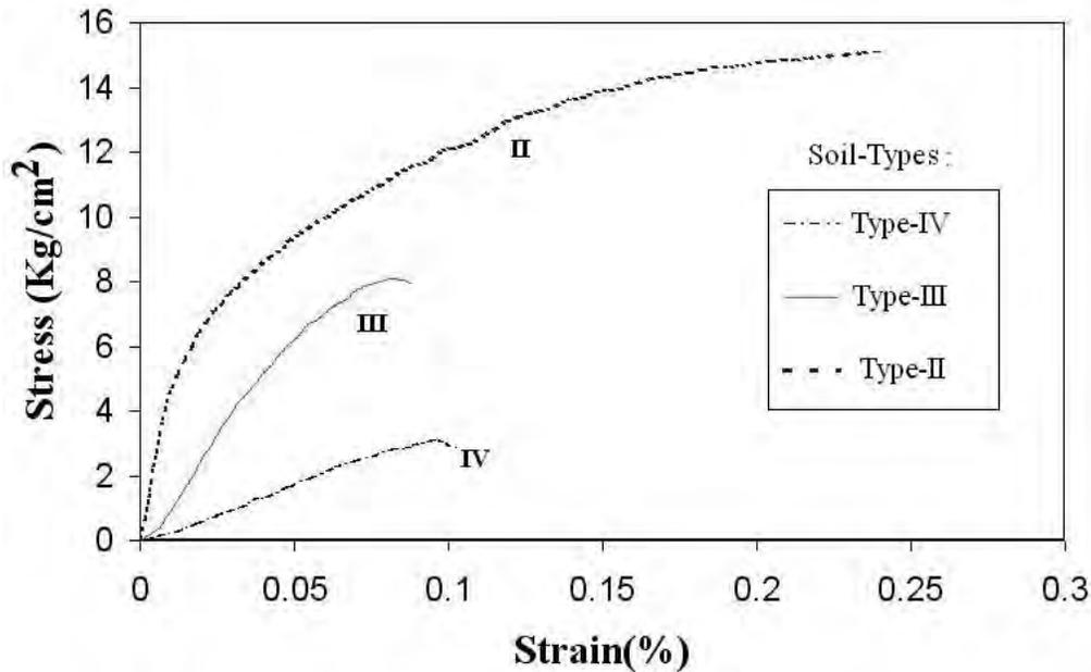
**Figure 7:** Stress-strain behavior of the Type-II, III, IV soil used for Analyses of SSI effect on Delijan's Silo
