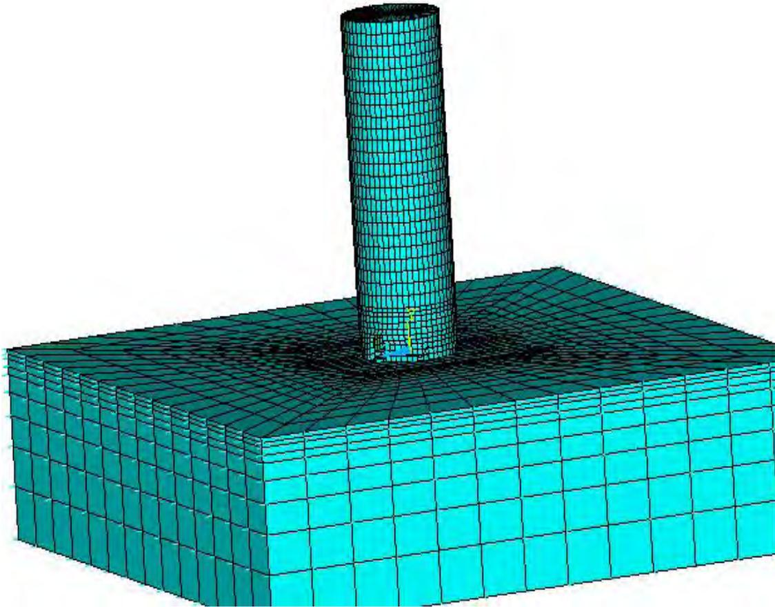
**Figure 3:** A Finite Element Model of Single Cell of Delijan's Silo Structure and its Foundation
