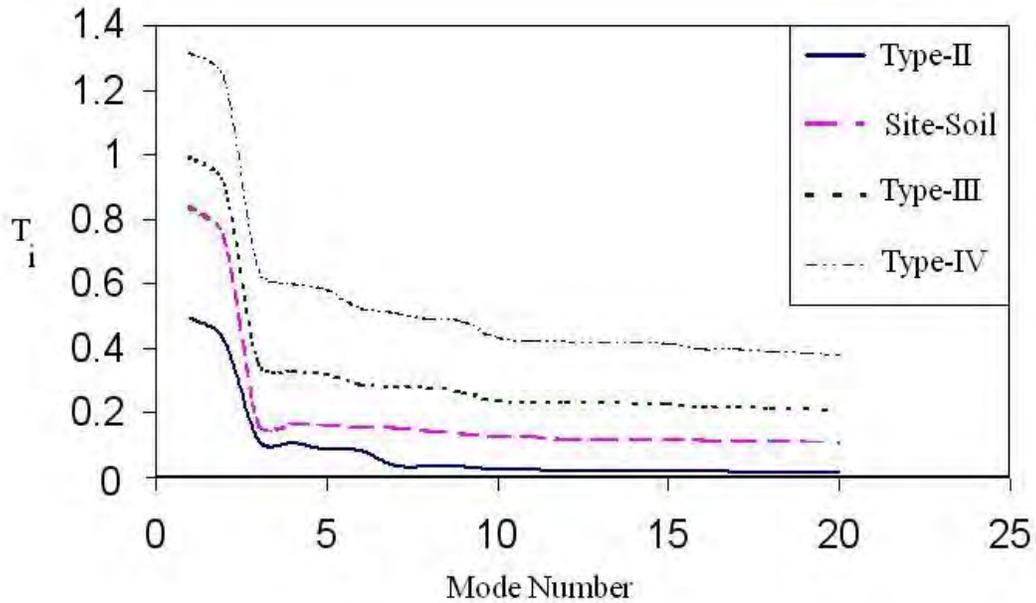
**Figure 12:** Variation of Modal Period vs. Mode Numbers for Delijan's Cement Silo with Various Supporting Soil Types
