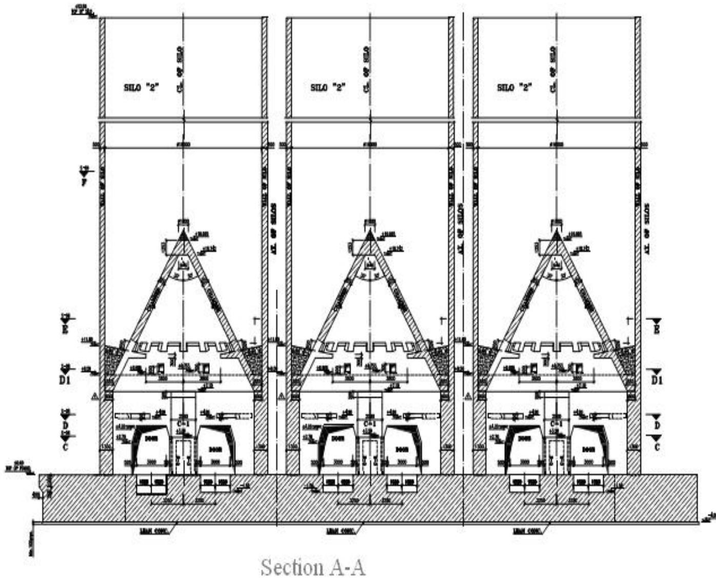
**Figure 1:** A Cross-sectional detail of Delijan’s cement storage Silo Structure and its Foundation
