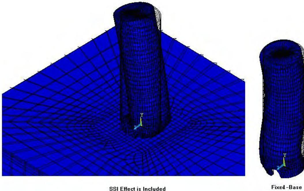
**Figure 9:** Shape of 8th Mode of Delija's Cement Silo System (SSI Effect vs. Fixed Base)
