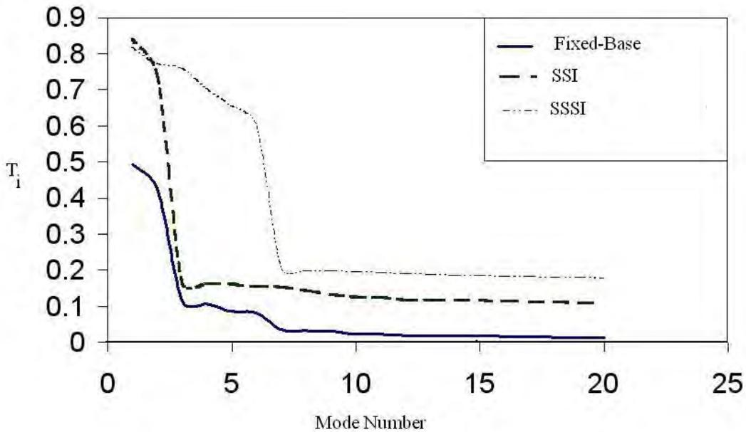
**Figure 13:** Variation of Modal Period vs. Mode Numbers for Delijan's Cement Silo with Various Support Conditions
