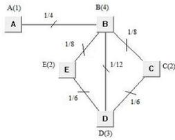
Figure 5. A sample network topology and weight of vertexes and edges in Parallel Connectivity Coefficient
