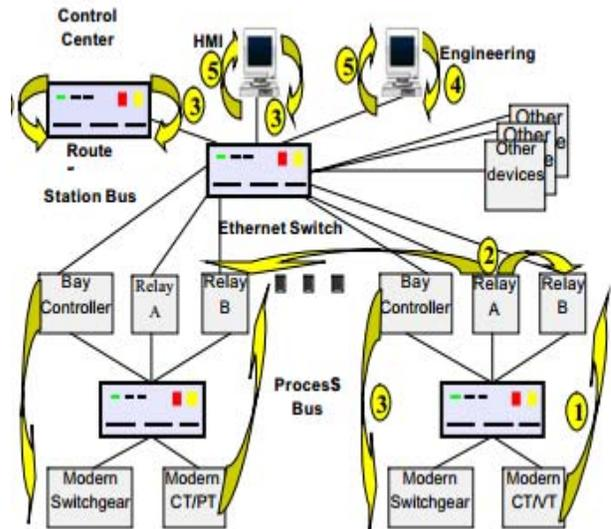
Figure 3. Conceptual substation automation topology
