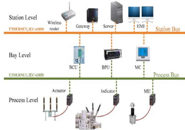
Figure 2. Substation automation layout
