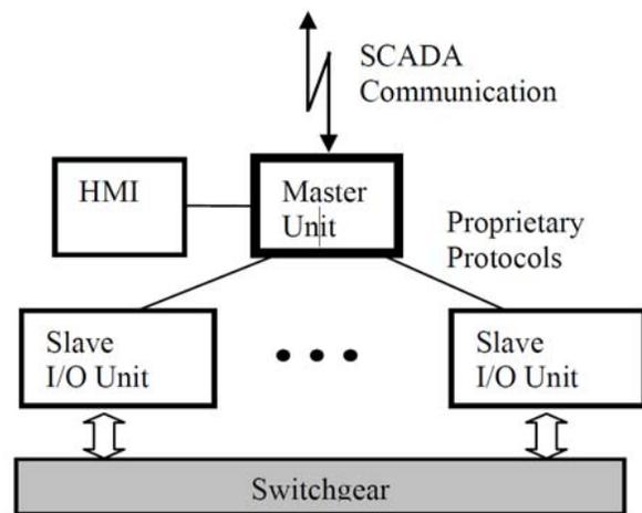
Figure 1. Initial architecture of a substation automation system
