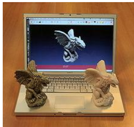
Figure 4.1: An example of real object replication by Means of 3D scanning and 3D printing
