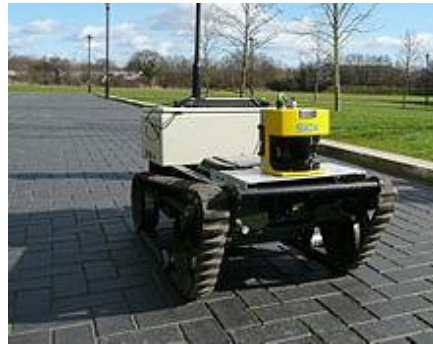
Figure 4.3: LiDAR-equipped mobile uses its LiDAR to construct a map and avoid obstacles
