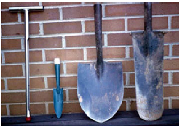
Figure 5. Some soil sampling tools.
