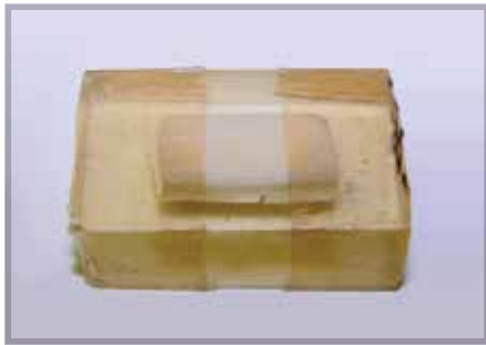
Fig 2. Polytetrafluoroethylene tape protecting both edges of the tooth specimen from acid erosion and serving as a reference area for analysis of surface loss.
